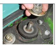
2 – Remove the rubber mount from the camber plate.
