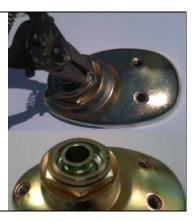
5 – Insert the shock through the Monoball cartridge assembly.
